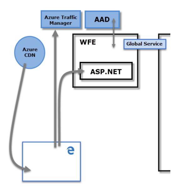
When users attempt to connect to the Power BI service, the client's DNS service may communicate with the **Azure Traffic Manager** to find the nearest datacenter with a Power BI deployment. For more information about this process, see <u>Performance traffic routing</u> <u>method for Azure Traffic Manager</u>.
